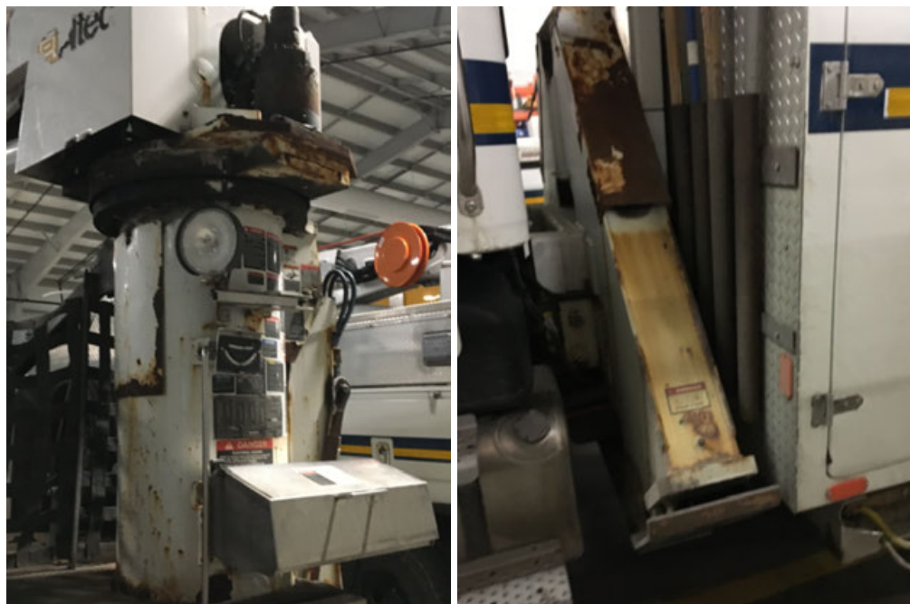
Figure 6 – Unit #2532 with Outrigger Structural Deterioration and Pedestal Corrosion 4
