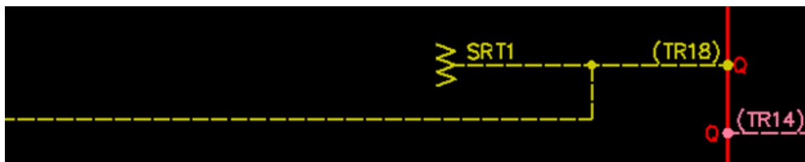
Figure 2.10- TR18 Breaker Supplying SRT1 13/4kV Transformer and Supply Feeder
