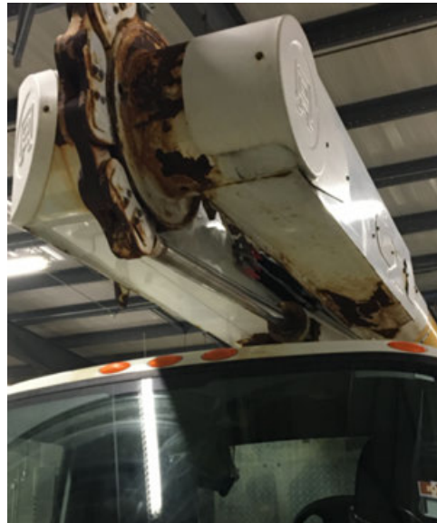
Figure 7 – Unit #2605 with Rust Deterioration on Boom
