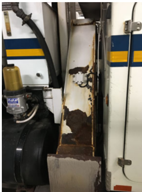
Figure 5 – Unit #2403 with Outrigger Structural Deterioration
