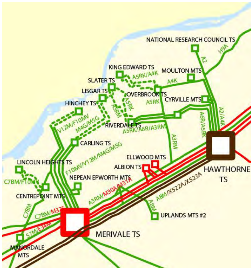
Figure 6-6: The 115 kV Transmission System in Ottawa
