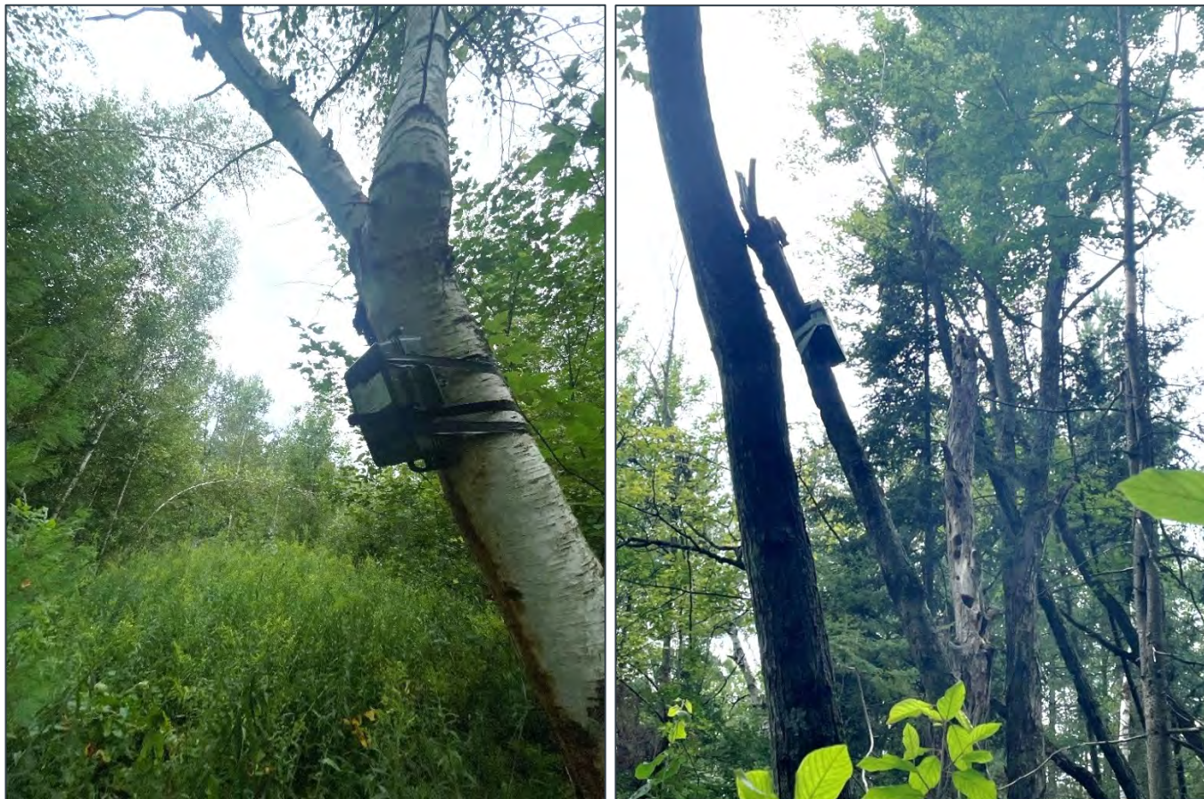
Photograph 1. Bat acoustical monitors deployed in edge habitat of the meadow and within the forest habitat, respectively.
