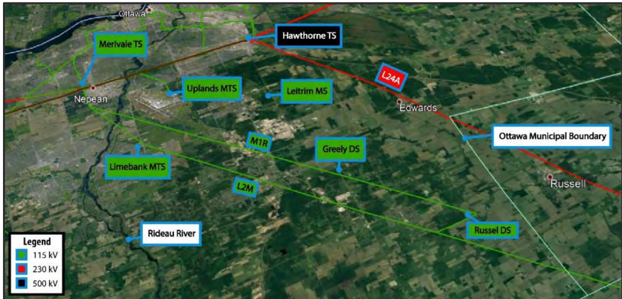
Figure 1 : Transmission System Layout in the Southeast Ottawa Area
