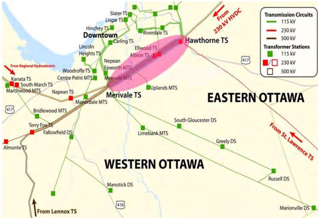
Figure 4-2: Hawthorne to Merivale Transmission Corridor
